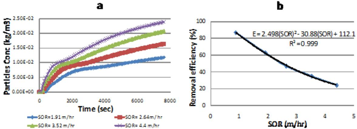
Fig. 6(a) Effect of SOR on the particles concentration at the outlet of the sedimentation basin
