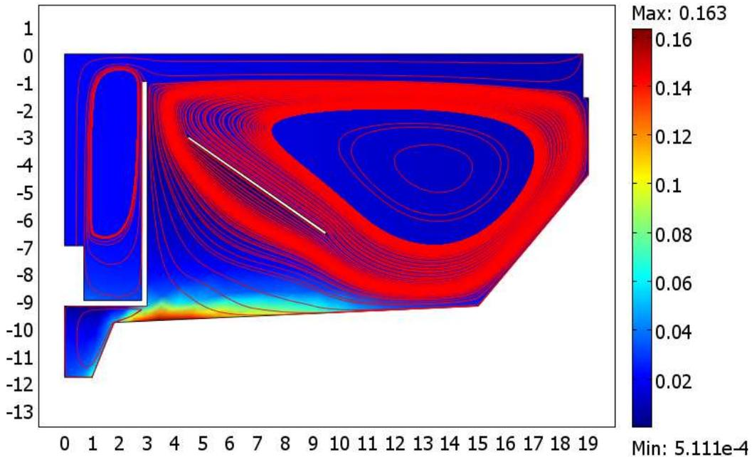
*Fig.3 Velocity streamline and settling behavior along the sedimentation basin*
