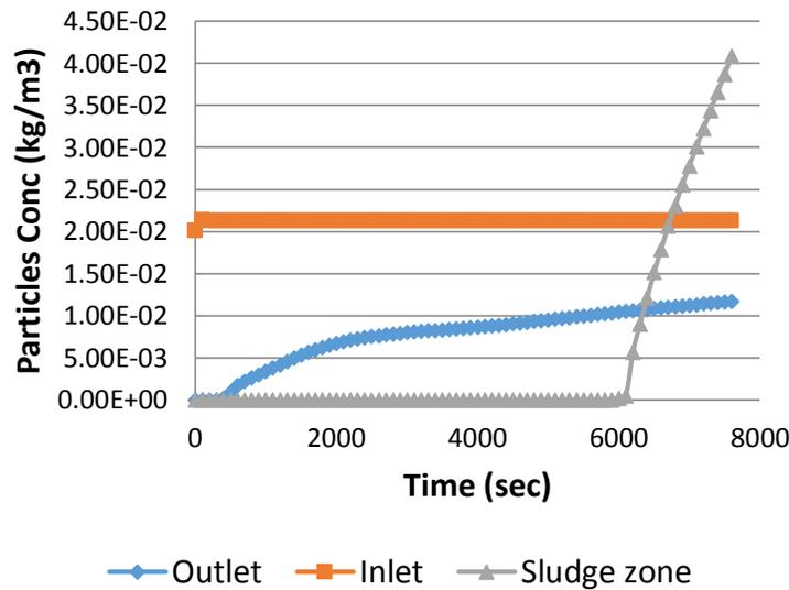
Fig.5 Comparison of the particle concentration at the inlet, outlet and sludge zones
