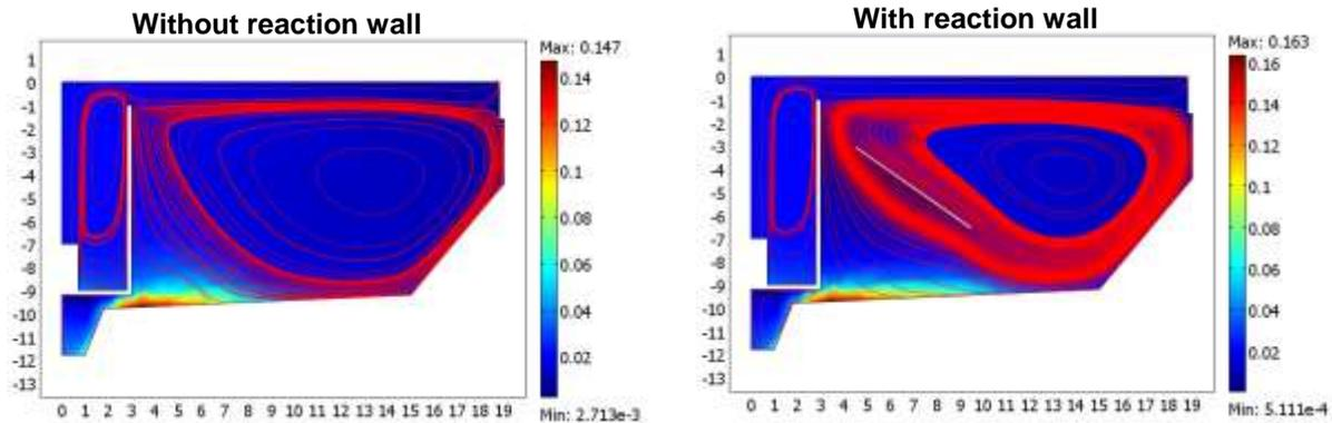
Fig.7 Effect of conical reaction wall on the flow and settling behaviors along the basin
