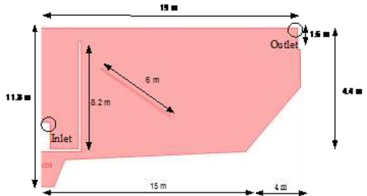
Fig. 2 Cross section of the half sedimentation basin
