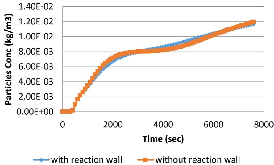
Fig.8 Effect of conical reaction wall on the particles concentration at the outlet of the sedimentation basin
